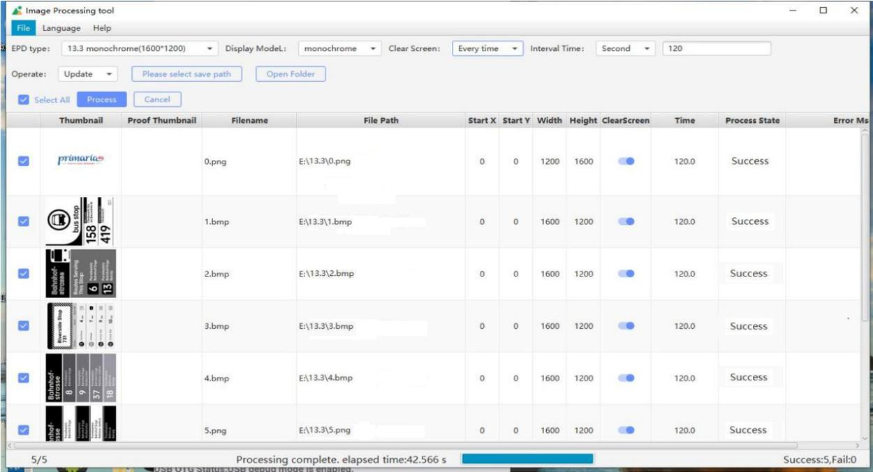
8. Once all images have been converted, you can click the "Open Folder" button in the software to view the created images. The created images will automatically generate an XT\_Resources folder, and the converted images will be saved in the image folder.
